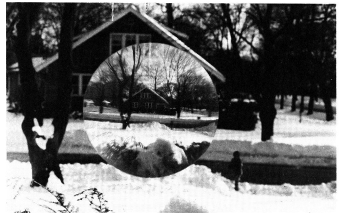
(d) The minified, rightside-up, virtual image formed by a negative lens.
